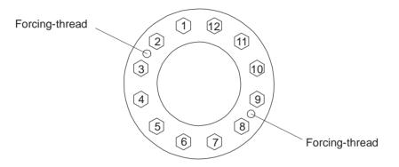
Figure 6.10.1-2: Sequence for tightening the clamping screws
