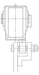
Figure 6.13.1: Torque arm on bevel helical gear unit
