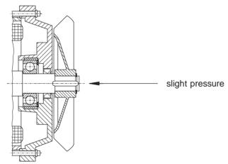
Figure 6.11.2-4: Pressure on motor shaft
