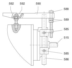
Figure 6.12.3: Mounting motor bedplate IEC motors from size 225
