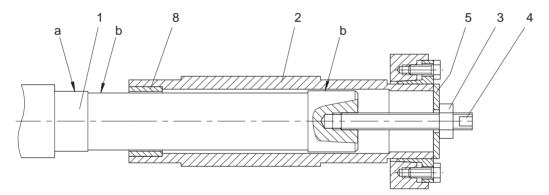
Figure 6.9.1-3: Mounting hollow shaft and shrink disk
