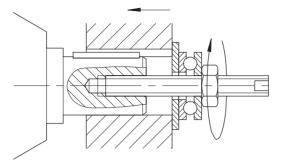
Example of a fitting device for fitting couplings or hubs on the ends of gear unit or motor shafts. If necessary, the axial thrust bearing on the fitting device can be dispensed with.
