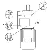
Figure 3.5.2-1: Mounting positions for D/Z38 - D/Z88
