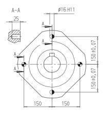
Figure 6.5–1: C-type housing flange helical gear units
