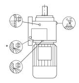
Figure 3.5.2-2: Mounting positions for D/Z108 - D/Z168
