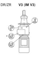
Figure 3.5.2-7: Mounting positions for DR/ZR68 - DR/ZR88
