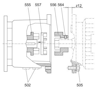
Figure 6.11.1: Coupling housing with torsionally flexible coupling
