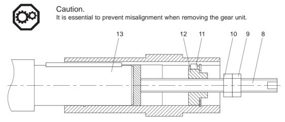
Figure 6.9.2: Remove hollow shaft and parallel key
