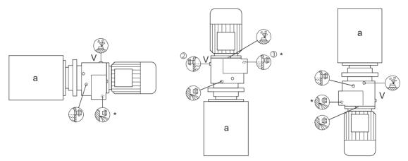
Figure 3.5.6: Operating position for dual gear unit
