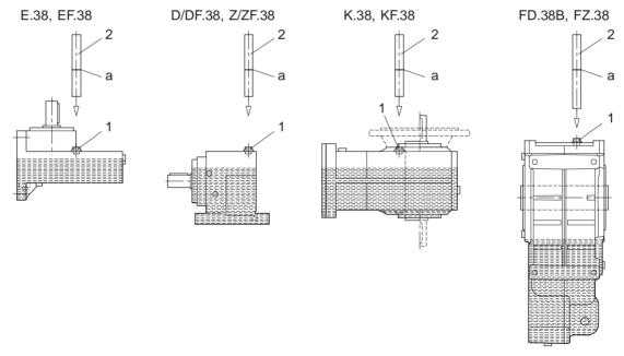
Figure 10.2.1.1-2: Oil level check on size 38 gear unit
