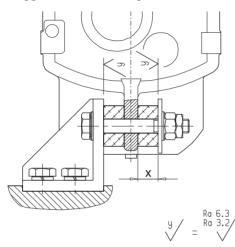
Figure 6.13.2: Torque arm on parallel shaft helical gear unit
