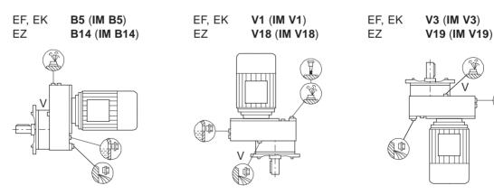
Figure 3.5.1–2: Mounting positions for E.38 - E.148
