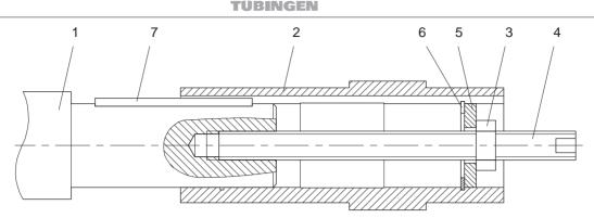
Figure 6.9.1–1: Mounting hollow shaft and parallel key
