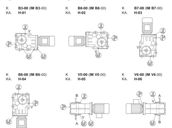
Figure 3.5.3–2: Mounting positions for K, KA, KAS, KAT Size 38 - 188
