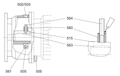
Figure 6.11.2-3: Coupling lantern with clamping ring
