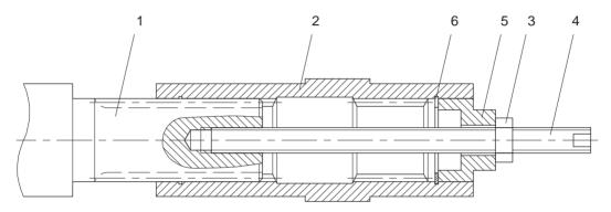
Figure 6.9.1-2: Mounting hollow shaft and splines
