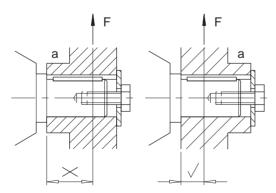
Correct mounting arrangement of running wheel, gear or chain wheel, belt pulley, etc., to keep the shaft and bearing load exerted by transverse forces as low as possible.
