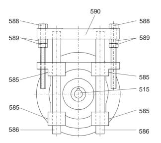
Figure 6.12.2: Mounting motor bedplate IEC motors sizes 132 to 200
