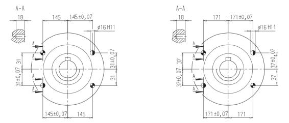
Figure 6.5-2: C-type housing flange bevel helical gear units and parallel shaft helical gear units
