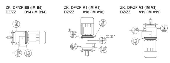
Figure 3.5.2–6: Mounting positions for D./Z.188
