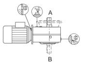
Figure 3.5.5-2: Mounting positions for CZ, CF, CAD, CAF, CAZ, CADS, CAFS, CAZS, CADT, CAFT, CAZT Size 38 - 88
